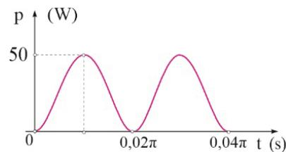
$$Q = I_{\text{ev}}^2 RT = \frac{I_{\max}^2}{2} RT \Rightarrow Q = \pi \text{ Joule}$$
