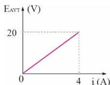
$$|E_{AYT}| = iR_{\text{ολ}} = i(R_1 + R_2) \Rightarrow |E_{AYT}| = 5i \text{ (SI)}$$
