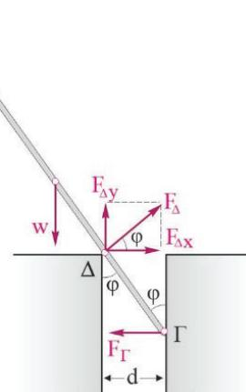
$$\text{Συνδυάζοντας τις (1), (2) παίρνουμε: } w \cdot \frac{L}{2} \eta \mu \varphi - \frac{w}{\eta \mu \varphi} (\Gamma \Delta) \Rightarrow w \cdot \frac{L}{2} \frac{1}{2} - \frac{w}{0,5} (\Gamma \Delta) \Rightarrow (\Gamma \Delta) = \frac{L}{8}$$
