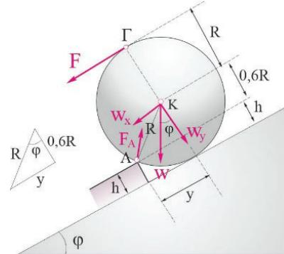
$$\Sigma \tau_{(A)} = 0 \Rightarrow F \cdot 1,6R + w \eta \mu \varphi \cdot 0,6R - w \sigma \nu \eta \varphi \cdot y = 0 , \quad (1)$$
