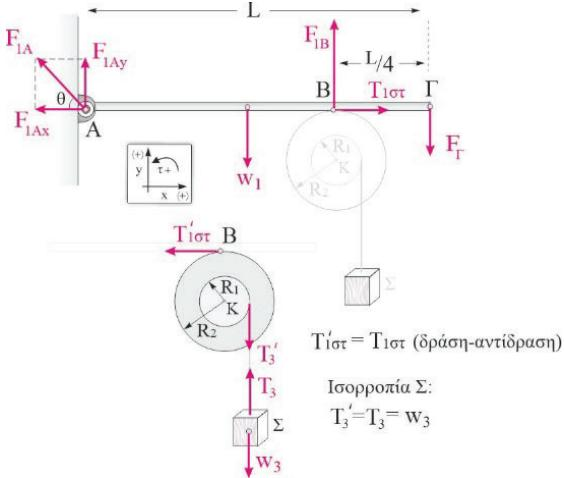
$$T'_{1\sigma\tau} = T_{1\sigma\tau} (\text{δράση-αντίδραση})$$
